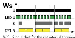
Ws) Single shot for the set interval triggered by closing of the control contact S.
