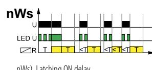
U - supply voltage; R - output state of the relay;
