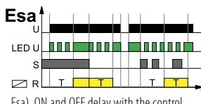
Esa) ON and OFF delay with the control contact S.
