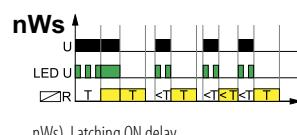
U - supply voltage; R - output state of the relay;
