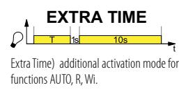
U - supply voltage; R - output state of the relay; S - control contact state; T - measured time; t - time axis
