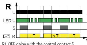
R) OFF delay with the control contact S.
