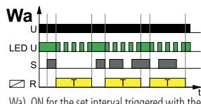
Wa) ON for the set interval triggered with the control contact S.
