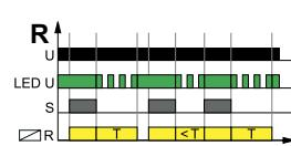
R) ON for the set interval controlled by closing of the control contact S, with the function of switching off the output relay R prior to the lapse of the interval T.
