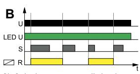
B) Cyclical operation controlled with closing of the control contact S.
